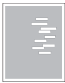
(2-14) Irregular horizontal white streaks appear in the image Dots appear in the image
