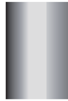
(2-8) Uneven density vertically
