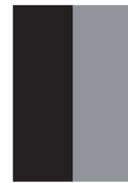
(2-8) Uneven density vertically
